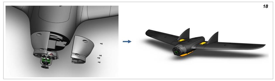
Check the cables assemble the right housing half. Secure with 4 screws
