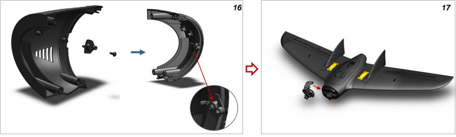
Mount pivot clip to left housing and secure with screw
