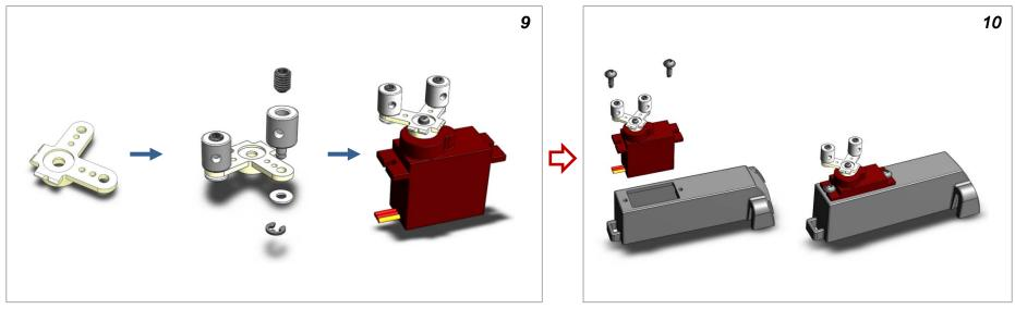
Assemble link stoppers to V-shaped servo horn secure with circlips (servo shall be centred)
