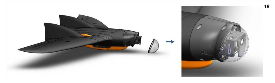
Finally attach the dome and rotate clockwise until it securely snaps into place. Congratulations, you have successfully assembled your RV-GoPro Pan & Tilt!
