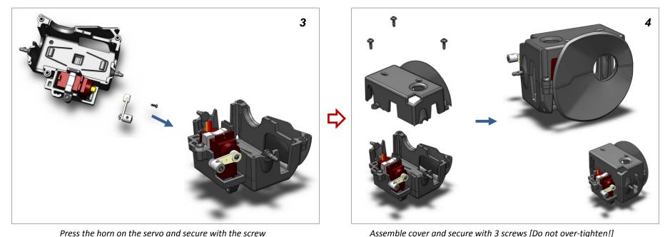
Assemble cover and secure with 3 screws [Do not over-tighten!] (In order to avoid scratches, do not insert GoPro yet)
