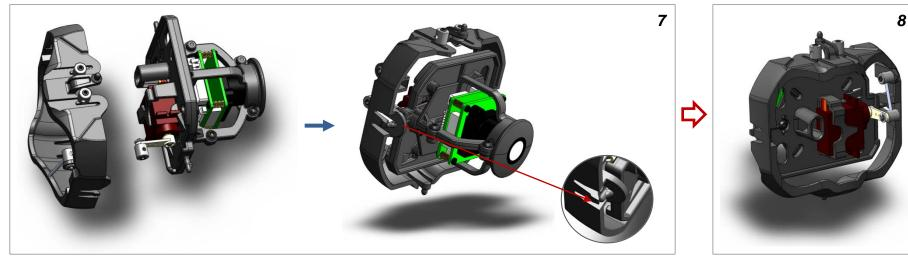
Snap camera assembly into ring. Do not to over-stress the snap features. Once into place it's very difficult to disassemble!
