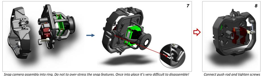
Snap camera assembly into ring. Do not to over-stress the snap features. Once into place it's very difficult to disassemble!
