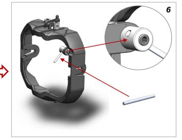
Assemble **18**mm push rod (flush with link stopper body)
