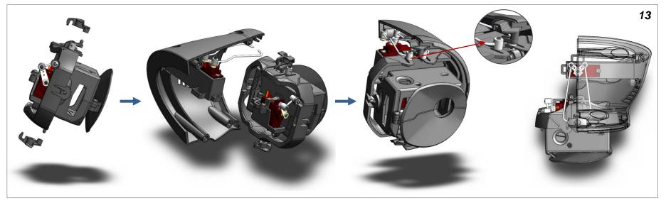
Attach the 2 pivot clips to the gimbal ring and insert into left housing. Insert the push rods into the link stoppers and tighten screws. Make sure everything turns smoothly.
