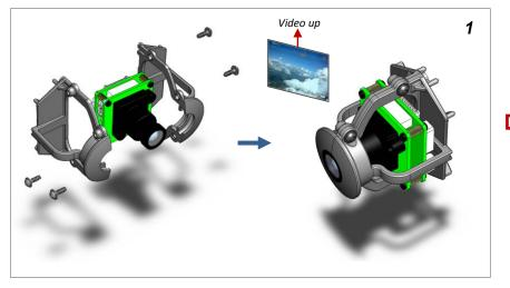
Mount your micro camera between the brackets and tighten the 4 screws (make sure the video orientation is correct!)
