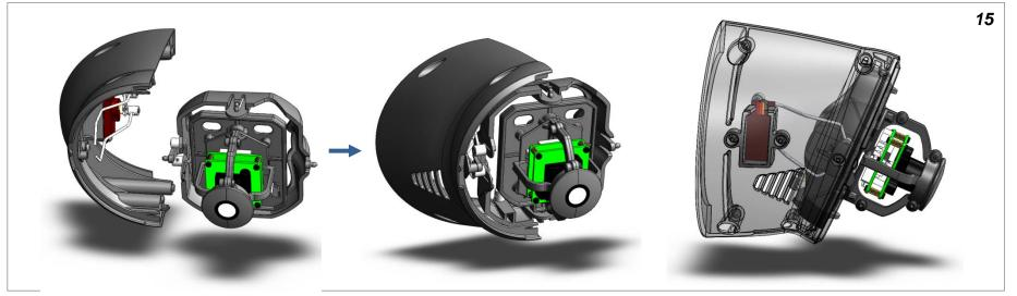
Insert the gimbal assembly into Right housing. Insert the push rods into the link stoppers and tighten screws. Make sure everything turns smoothly.
