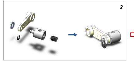
Assemble link stopper on servo horn and secure with circlip
