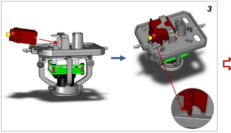
Push the servo in place until the 2 snap fits lock into place
