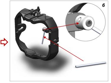
Assemble **26**mm push rod (flush with link stopper body)
