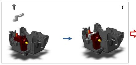
Mount servo and secure with clip and screw [Do not over-tighten!]
