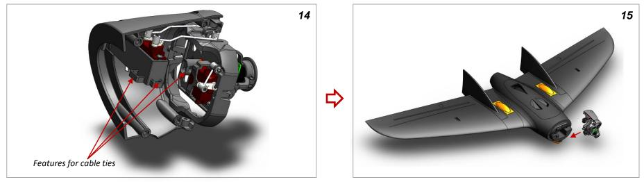
Route the servo and video cables and fix them with small cable ties to the provided features (make sure you allow enough slack for movement!).
