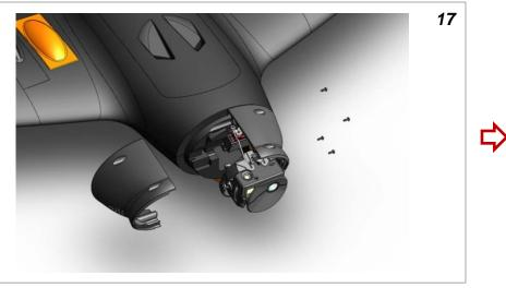
Re-check the cables assemble the right housing half. Secure with 4 screws
