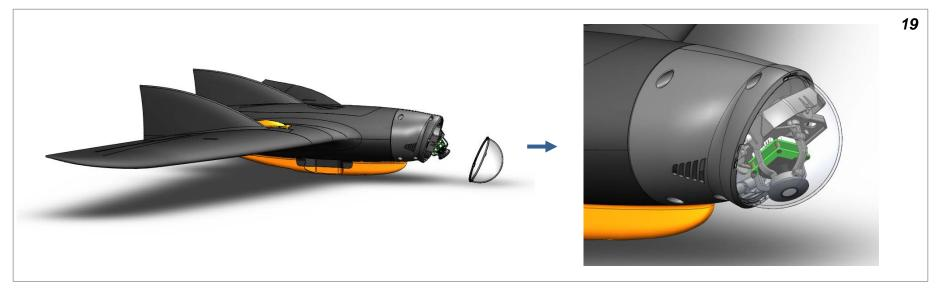
Finally attach the dome and rotate clockwise until it securely snaps into place. Congratulations, you have successfully assembled your RV-MiniCam Tilt & Pan!
