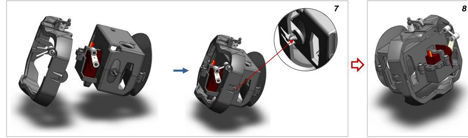
Snap GoPro holder into ring. Make sure not to over-stress the snap features. Once into place it's very difficult to disassemble!
