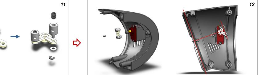
Align horn according to picture (parallel with front edge) and push onto servo. Secure with screw. The servo should be centred prior to this step
