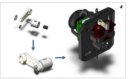
Assemble link stopper on servo horn and secure with circlip Push horn on servo an secure with screw as shown (servo shall be centred)
