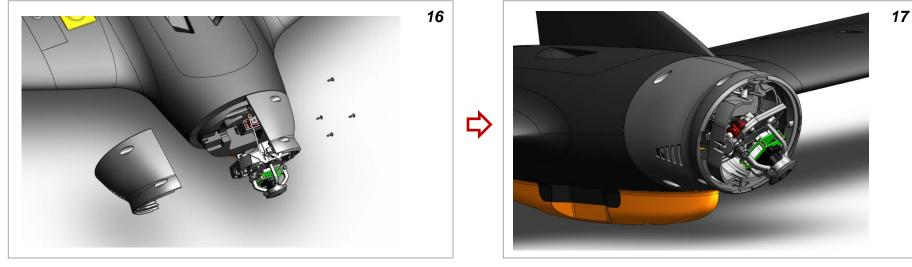
Re-check the cables assemble the right housing half. Secure with 4 screws
