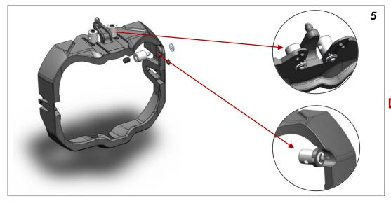
Assemble 3 link stoppers to gimbal ring and secure with circlip according to picture (please note which holes are used)
