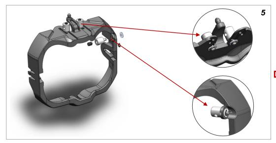
Assemble 3 link stoppers to gimbal ring and secure with circlip according to picture (note which holes are used)
