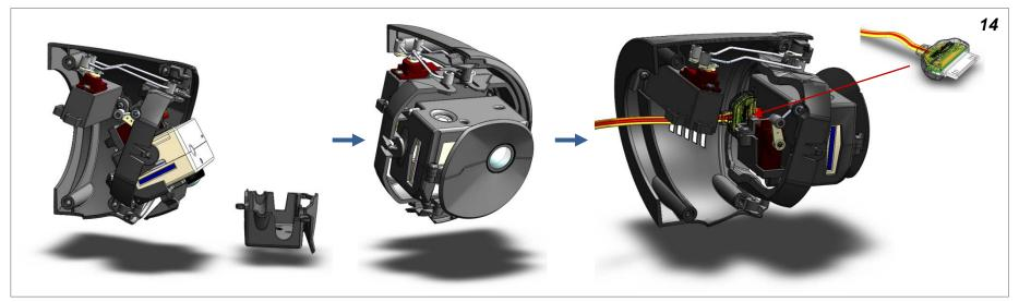
Now remove the GoPro cover and insert your GoPro. Insert the (optional) Range Video GoPro connector for live video-out and in-flight charging. Remount the cover.
