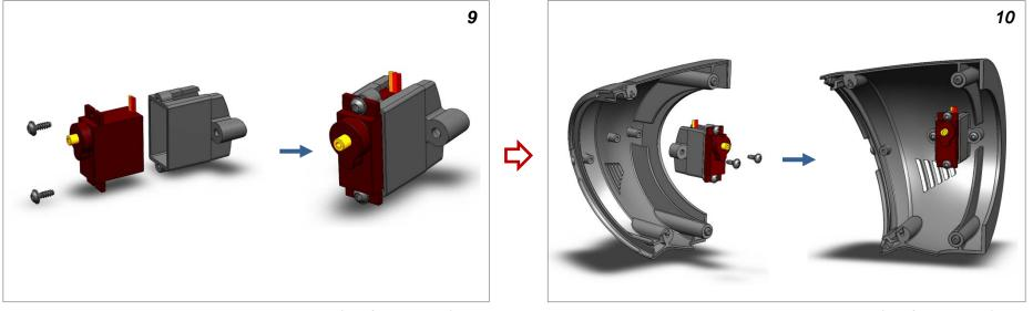
Insert servo holder and secure with 2 screws (careful with cable)
