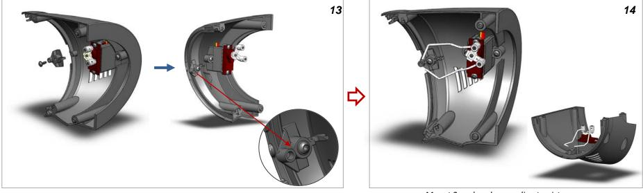
Mount pivot clip to right housing and secure with screw
