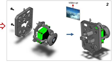
Push assembled camera bracket onto base plate and insert 2 screws (Note the video orientation!)
