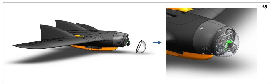
Finally attach the dome and rotate clockwise until it securely snaps into place. Congratulations, you have successfully assembled your RV-MiniCam Pan & Tilt!
