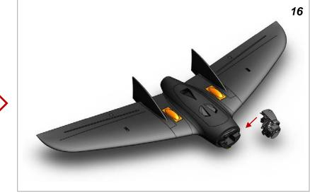
*Slide the complete assembly carefully onto the RV-JET fuselage.*
