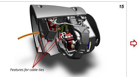
Route the servo and video cables and fix them with small cable ties to the provided features (make sure you allow enough slack for movement!).
